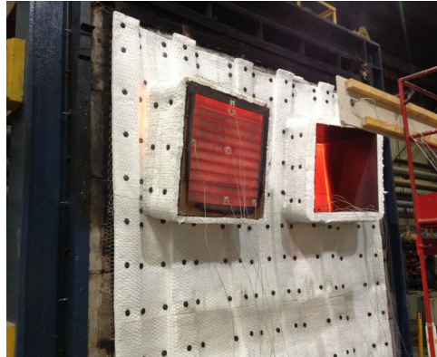
Actual Hydrocarbon Fire Test in an H60 Steel Bulkhead
